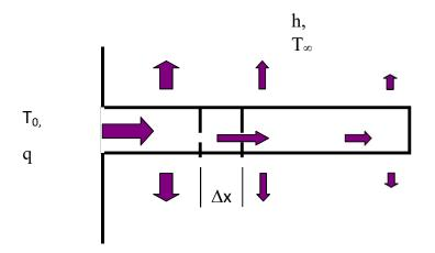
Across this segment the heat loss will be  $h \cdot (P \cdot \Delta x) \cdot (T - T_{\infty})$ , where P is the perimeter around the fin.
