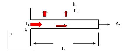
The fin is situated on the surface of a hot surface at  $T_s$  and surrounded by a coolant at temperature  $T_{\infty}$ , which cools with convective coefficient, h. The fin has a cross sectional area, A<sub>c</sub>, (This is the area through with heat is conducted.) and an overall length, L.
